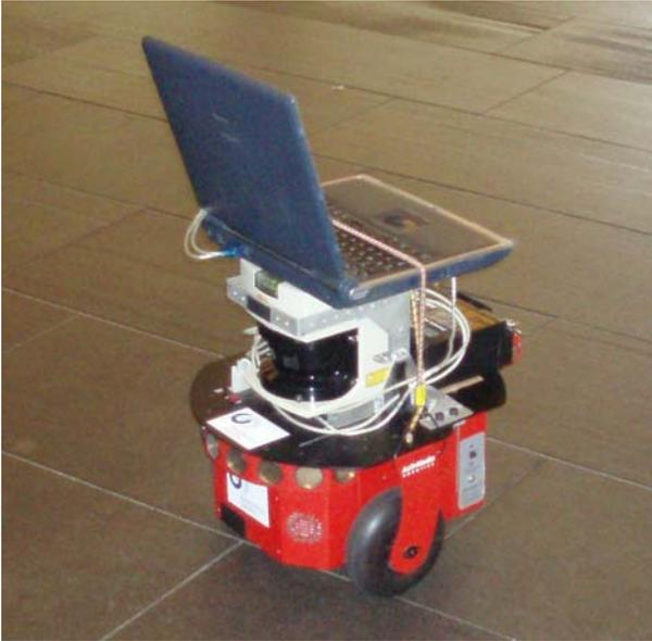
Figure 4: Pioneer 2DX used for LAM and PPOA development.
