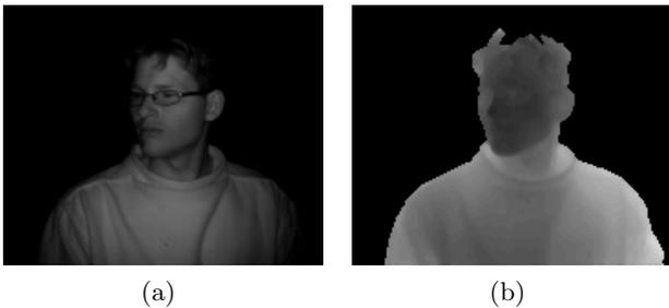
Figure 2: (a) Sample SR-3000 amplitude image, and (b) corresponding depth map
