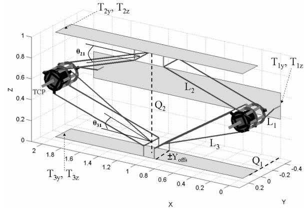
Figure 5: The 3-DOF reconfigurable Gantry-Tau robot.
