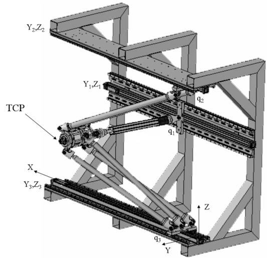
Figure 6: A prototype of the 3-DOF Gantry-Tau with a triangular-mounted link pair.
