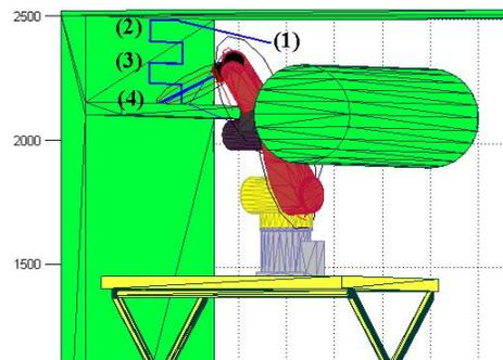
Figure 6. A case study in a complex blasting environment [Chotiprayanakul, Liu, et al., 2007b]
