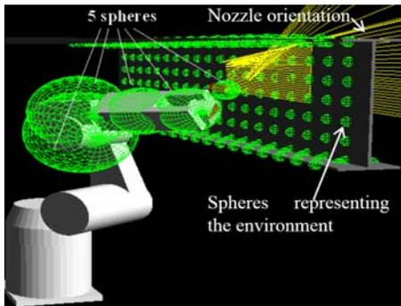
Figure 4. Spheres enclosing the robot arm and the environment can be used in collision avoidance. [Xu, Liu, et al., 2007]
