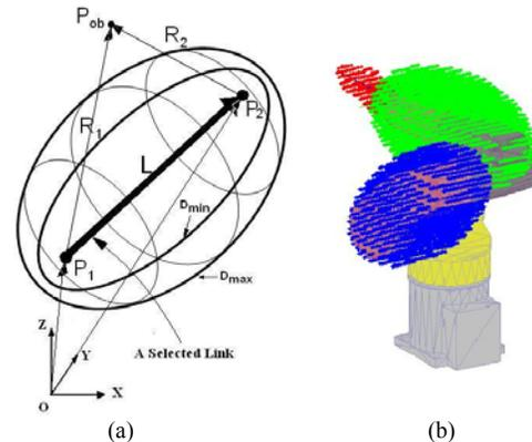
Figure 5. (a) Definition of a 3D force field; (b) A robot arm covered by a 3D force field [Chotiprayanakul, Liu, et al., 2007a]
