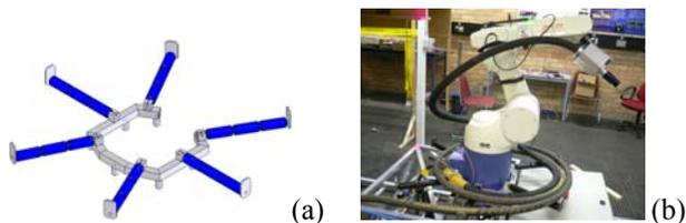
Figure 9. A roller arm assembly for blast hose management [Robertson, 2008]
