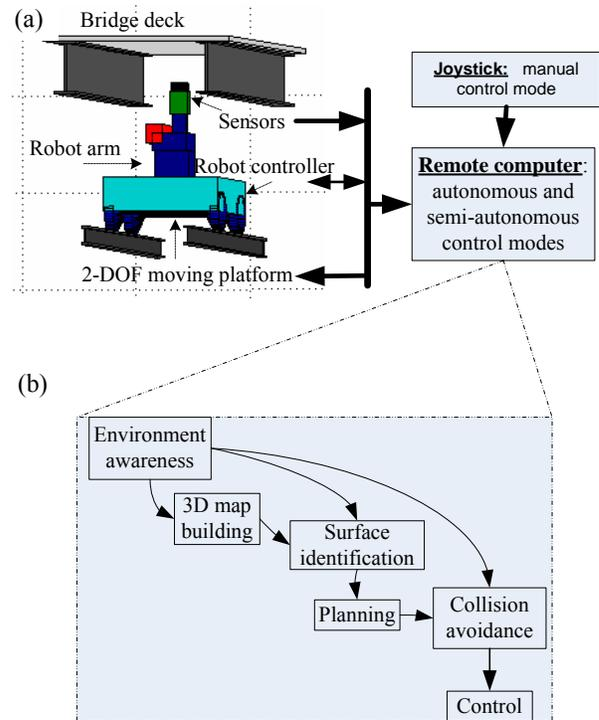
Figure 1 (a) System architecture of an autonomous robotic system for grit blasting in bridge maintenance; (b) Key components and the flowchart
