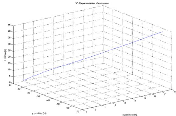
Figure 19: Gyroscope drift
