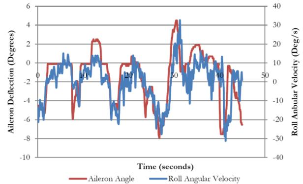
Figure 18B: Roll angular velocity response
