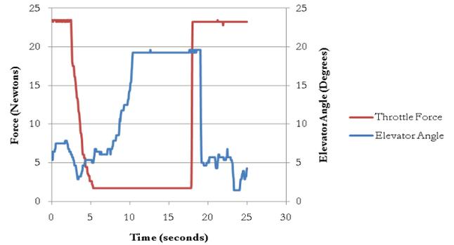
Figure 14: Control inputs for throttle variation manoeuvre
