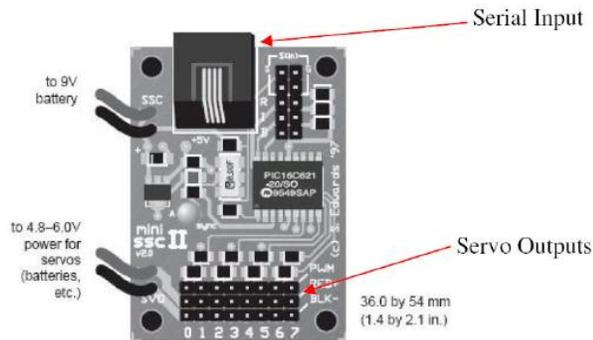
Figure 8: Serial Servo Controller
