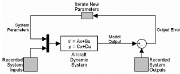
Figure 5: Parameter estimation iterative process
