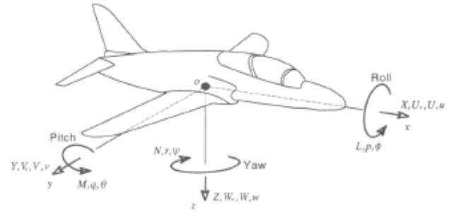
Figure 2: Aircraft body axes coordinate system [Cook, 1997]
