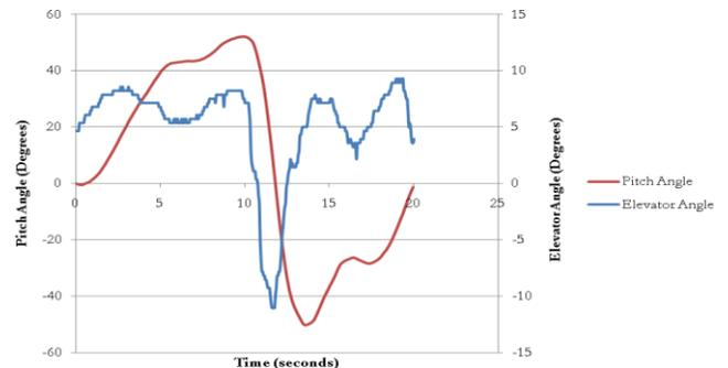
Figure 13: Pitch angle for the pull up-push over manoeuvre
