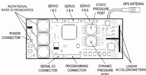
Figure 6: Inertial Measurement Unit board layout
