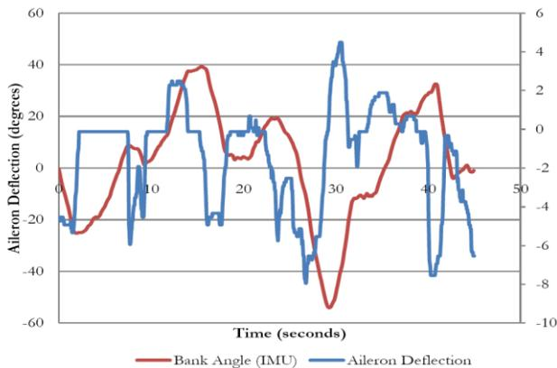
Figure 18A: Bank angle for 'figure of eight' manoeuvre
