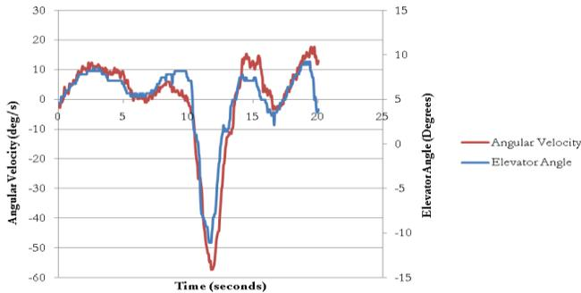
Figure 17: Pitch angular velocity response
