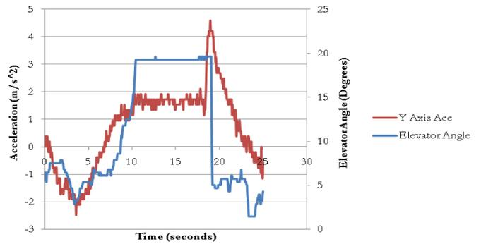
Figure 15: Stall conditions creating Y axis acceleration
