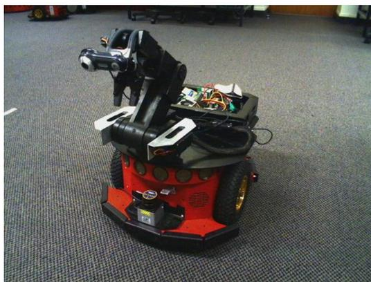
Figure 3: Pioneer 3DX robot with a camera mounted on the robot arm
