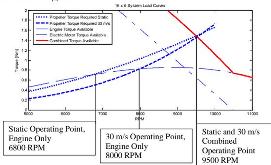
Figure 1.7 Hybrid Powerplant Experimental Results Load Curves
