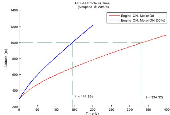
Figure 2.1 Simulated AHP Boosted versus Non-boosted Climb Performance
