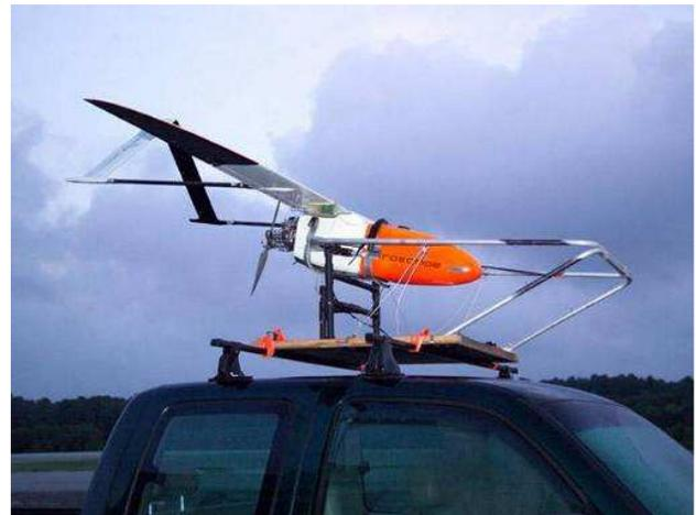
Figure 1.6 Aerosonde Launch Mechanism
