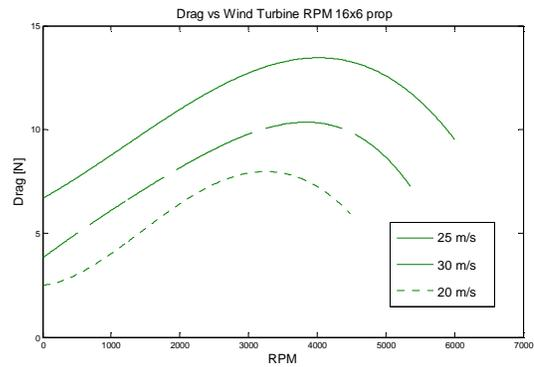
Figure 2.4 Propeller Turbine Drag
