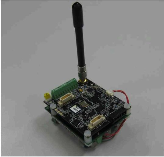
Figure 1: Fleck 3 Wireless Sensor Node. The size of main board is 50x60mm.
