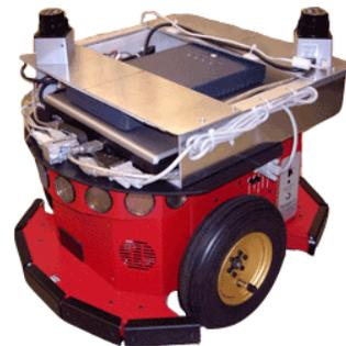
Figure 1 – Pioneer P3DX Mobile robot with front and rear Hokuyo URG laser range finders.
