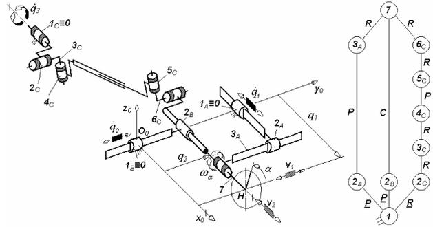
Figure 1.  $\underline{PPR}\text{-}\underline{PC}\text{-}\underline{RUPU}$ -type basic solution of maximally regular T2R1-type PM
