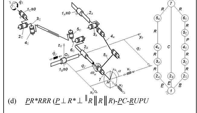
Table 4. Kinematic structures of maximally regular  $T2R1$ -type spatial PMs with one degrees of overconstraint derived from the basic solution  $\underline{P}RRR-PC-\underline{R}UPU$  by combining one idle mobility in limb  $G_1$  (a-b) or in limb  $G_2$  (c-d)
