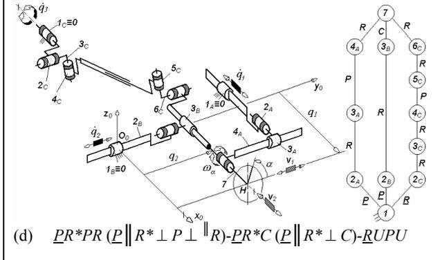
Table 3. Kinematic structures of maximally regular  $T2R1$ -type spatial PMs with one degree of overconstraint derived from the basic solution  $\underline{P}PR-PC-\underline{R}UPU$  by combining one idle mobility in each limb  $G_1$  and  $G_2$
