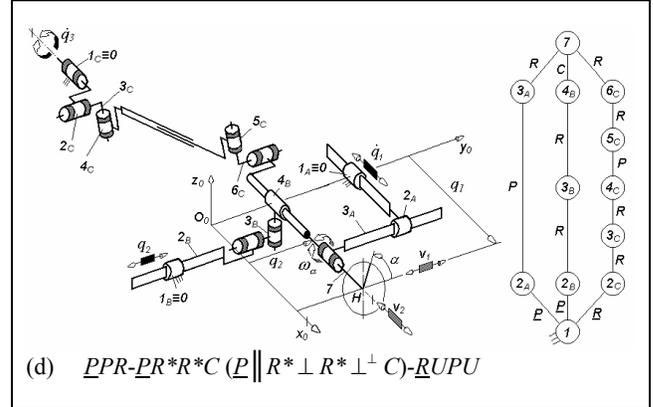
Table 1. Kinematic structures of maximally regular  $T2R1$ -type spatial PMs with two degrees of overconstraint derived from the basic solution  $\underline{PPR}\text{-}\underline{PC}\text{-}\underline{RUPU}$  by combining one idle mobility in limb  $G_1$  (a-b) or in limb  $G_2$  (c-d)
