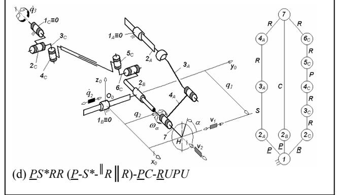
Table 7. Kinematic structures of non overconstrained maximally regular  $T2R1$ -type spatial PMs derived from the basic solution  $\underline{PR}^*C^*R$ - $\underline{PC}$ - $\underline{RUPU}$  by combining three idle mobilities in limbs  $G_1$  and  $G_2$  (a-c) or just in limb  $G_1$  (d)
