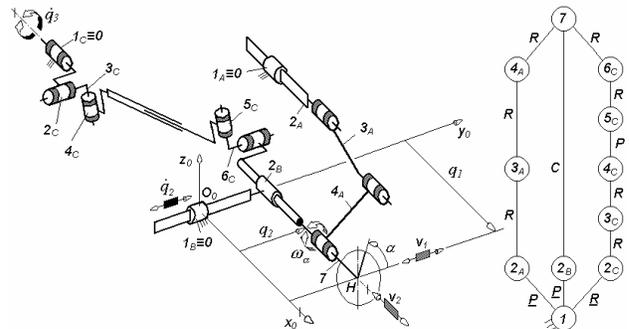
Figure 2.  $\underline{PRRR}\text{-}\underline{PC}\text{-}\underline{RUPU}$ -type basic solution of maximally regular T2R1-type PM
