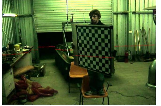
Figure 3: Laser scan drawn in image frame: Illustrates calibration quality of offset and rotation between camera and laser frames
