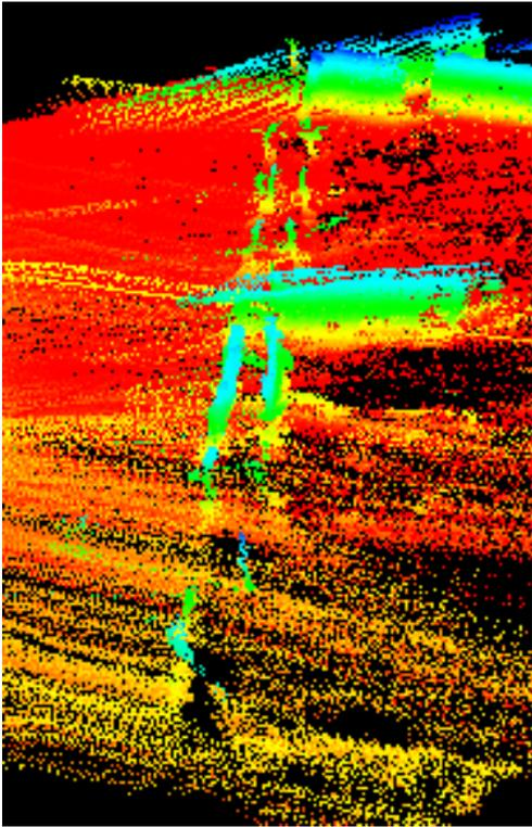
Figure 4: Yaw between laser and navigation system uncalibrated. Scan of fence single fence line appears duplicated in map
