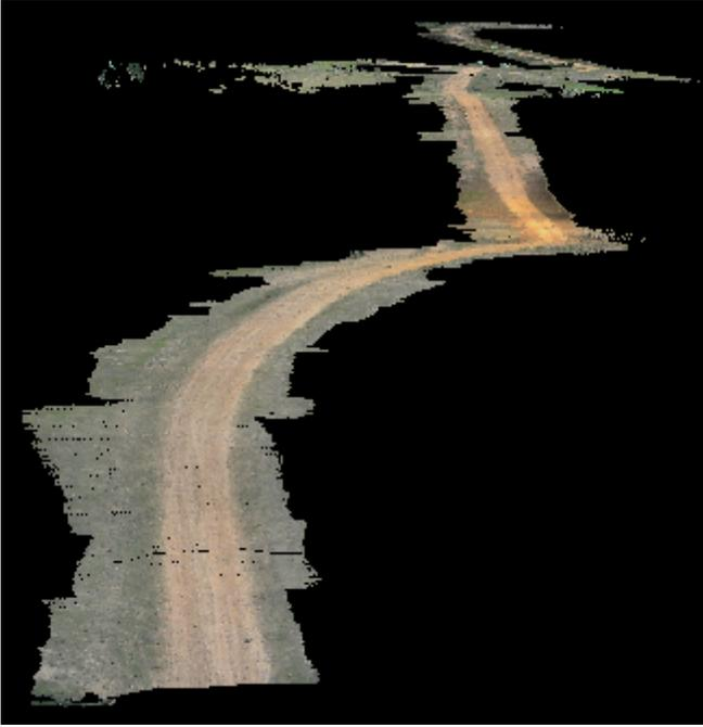
Figure 8: Colour map of dirt road. Mean locations plotted as a point cloud with colour. Colour mapping preserves visual texture of the ground. Only points in the field of view of both the laser and camera are shown.
