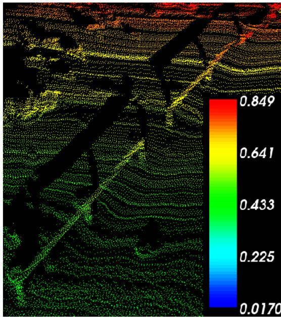
Figure 7: View of road-side fence coloured by uncertainty as largest orthogonal standard deviation in metres, calculated by equation 12.
