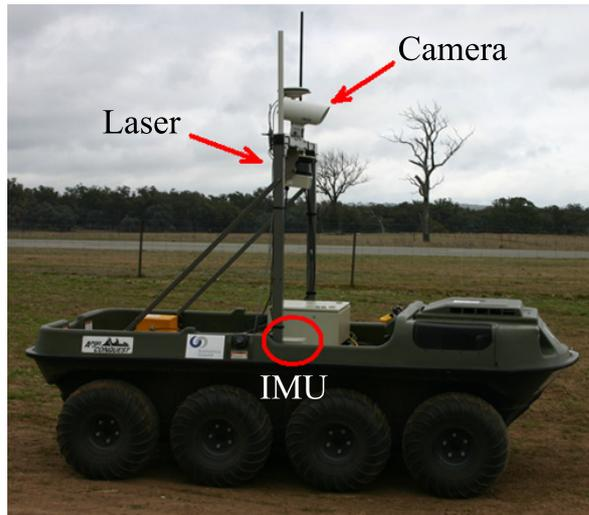
Figure 1: Photo of autonomous ground vehicle showing locations of laser scanner, colour camera and Inertial Measurement Unit (IMU)
