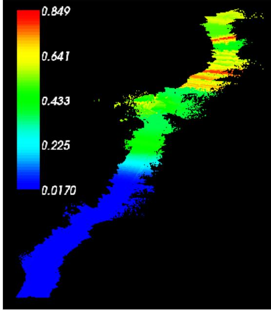
Figure 6: Map of dirt road coloured by uncertainty as largest orthogonal standard deviation in metres, calculated by equation 12.
