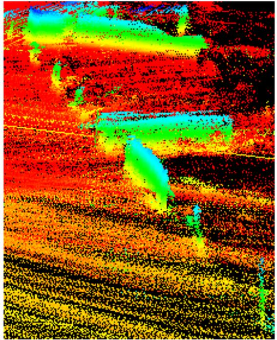
Figure 5: Yaw between laser and navigation system calibrated correctly. Scan of single fence line appears as a single focussed fence line in map
