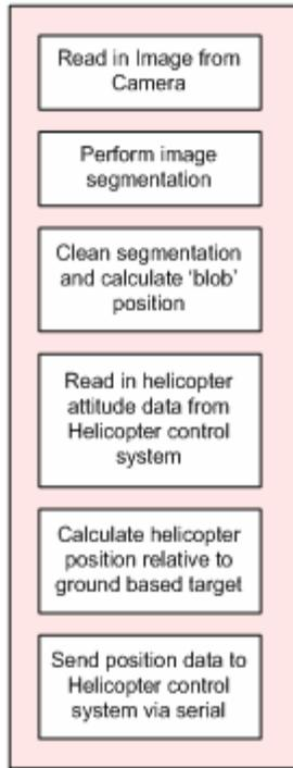
Figure 6 – Flow of Vision System Software
