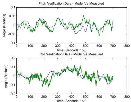
Figure 10 - Verification of Helicopter Model
