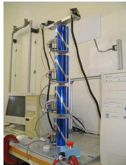
Figure 12. Four Module Assembled Manipulator System
