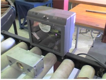
Fig.5. The PSC VS1200 barcode reader used for part identification
