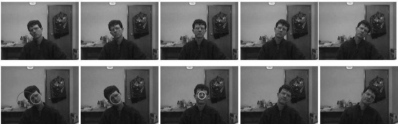
Figure 10. (Top) Classifier based on standard features in a Viola-Jones classifier fails when given large ( 45^\circ ) in plane rotations. (Bottom) Using two rotated Viola-Jones classifiers (shown using orange and red) and one standard Viola-Jones classifier (shown using yellow) the face can be identified both with and without in plane rotations. Note: as shown in the bottom left image some spurious face candidates are intermittently identified, some of these can be filtered out using the candidate faces from a sequence of images in a video.
