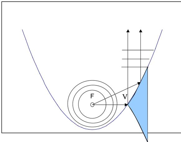
Figure 1 - Parabola with focal point F. A point source at F will result in circular wave fronts emanating from the focus F that when reflected by the parabola become plane wave fronts. The slope at V is 1. The shaded (blue) region is the cross section of the cone used as a reflector in this paper.
