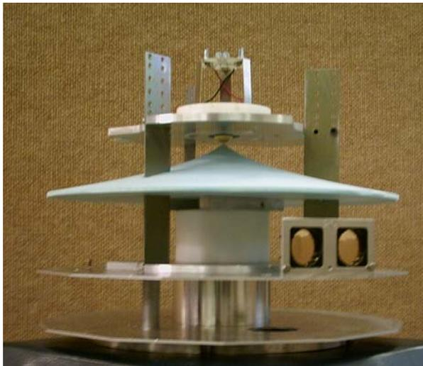
Figure 2 - The machined parabolic cone of diameter 300 mm mounted below the transmitter described later in the paper. Two Polaroid 7000 series transducers are shown below the reflector that will be part of the 48 receivers planned for the sonar ring.
