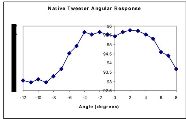
Figure 12 Measured Tweeter Response to 2 Cycles 65 Volts 45 kHz peak to peak versus angle from axis.
