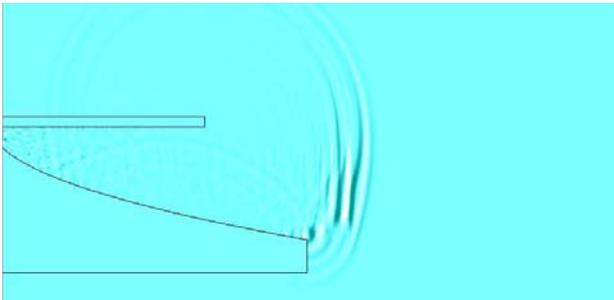
Figure 6 – Diffraction from the bottom reflector terminatin evident.
