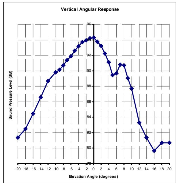
Figure 13 - Measured sound pressure level dB for differing elevation angles for the parabolic cone – transducer combination. Positive angle is above the transmitter. Two cycles of 45 kHz is emitted from the ESTD Murata tweeter and the measured sound pressure level is reported.
