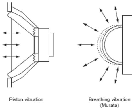
Figure 10 - Cross sectional comparison of vibration of a piston versus the ESTD “breathing” vibration – taken from [Murata 2006].
