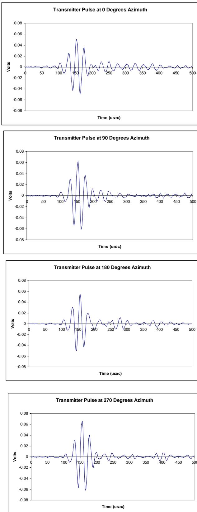
Figure 14 – Final Design of reflector and transmitter pulse shapes at different angles around the sonar ring.
