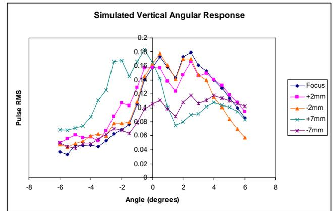
Figure 8 – RMS pulse amplitude versus vertical angle from the reflector at 1 metre for varying distance between the point source and the tip of the reflector.
