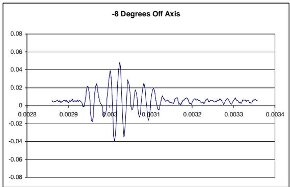
Figure 11 - Off axis free air response of the ESTD01 transducer with its housing removed. Measurements taken with Bruel Kjaer Cartridge type 4135 ¼" condenser microphone with the ESTD01 driven with 2 cycles of 45 kHz at 65 Volts peak to peak. The time axes are in seconds and the vertical axis is in Volts. All measurements were taken at 1 metre with the microphone on +20dB setting.
