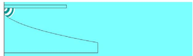
Figure 3 – The commencement of a TLM simulation of the conical reflector. The transmitter is modelled as a point source with a reflector immediately behind it near the top left of the simulation. Light areas are of high pressure and
