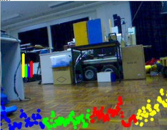
**Figure 10** K-means clustering of columns based on number of leg-coloured pixels in each column. Cluster count is fixed to four. Mean values of clusters are displayed as vertical bars
