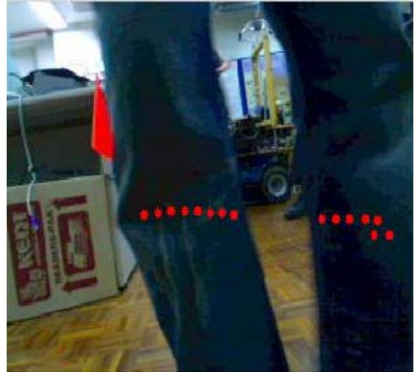
Figure 5 Laser leg segments projected onto image
