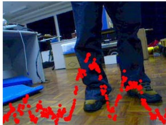
**Figure 8** Plot of number of leg-coloured pixels in each column of the image
