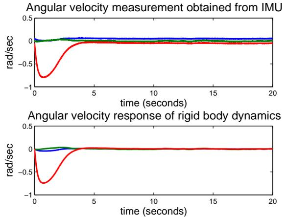
Figure 2: The evolution of the IMU measured values (top) and the true values of angular velocity for the rigid body dynamics. Note that the measured values in the top graph show a constant bias. This is compensated for the combined control design.
