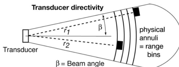
Fig 12 K-sonar CTFM transducer
