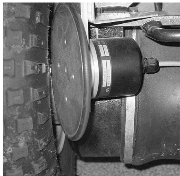
Fig 8 Encoder driven by rear wheel through friction coupling.
