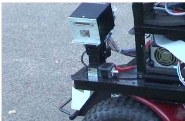
Fig 10 Titan's Sonar array pan and tilt mounting
