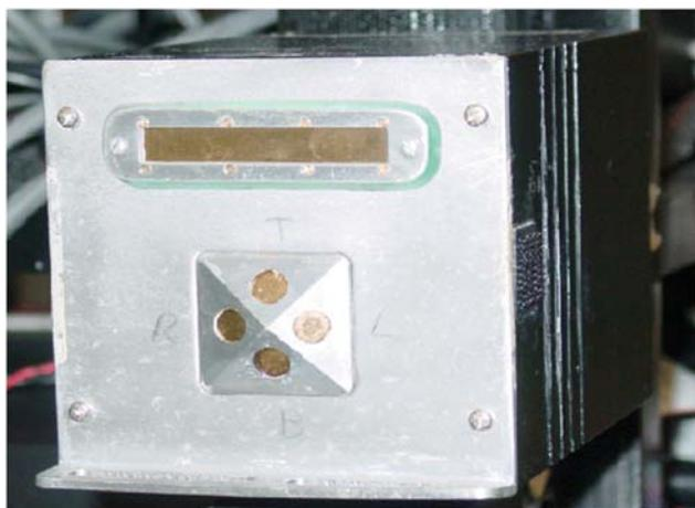
Fig 9 Titan's Sonar array
