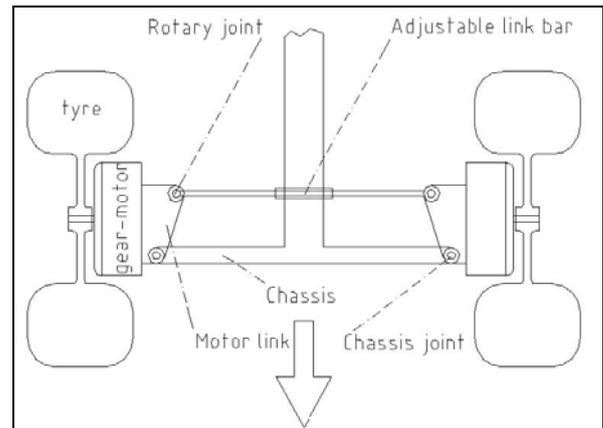
Fig 7 Titan's steering assembly
