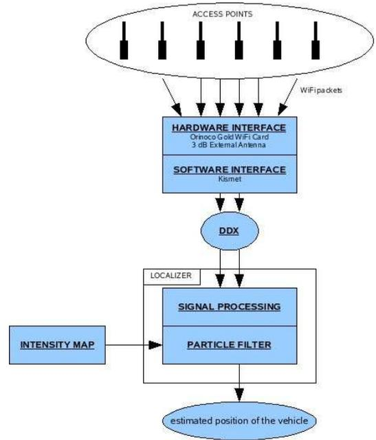
Figure 7: Architecture of the system.
