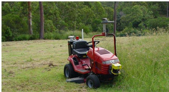
Figure 1: Our tractor lawn mowing vehicle autonomously cutting long grass.
