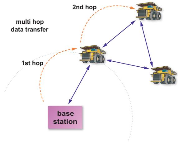
Figure 2: The mesh network allowing multihop data transfer
