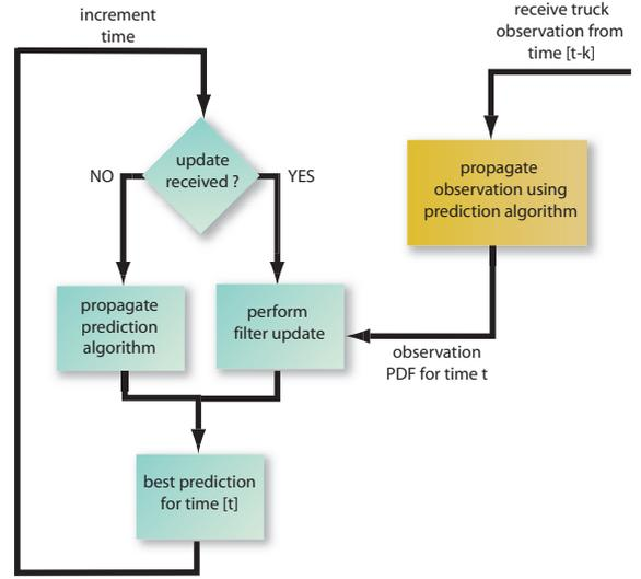
Figure 5: Overview of the Filter/Prediction algorithm
