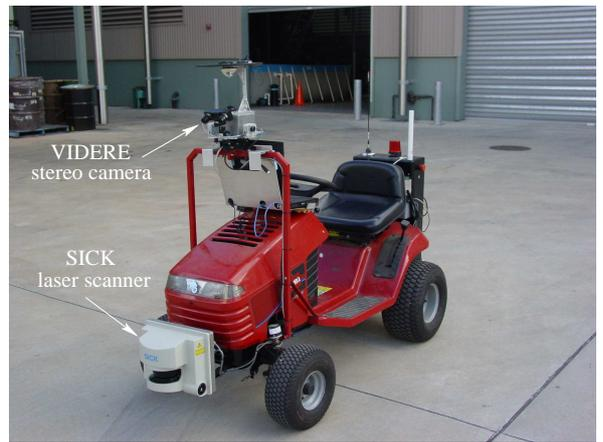
Figure 1: The Autonomous Tractor highlighting the sensors used in these experiments.
