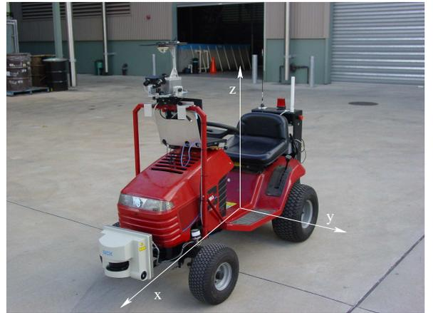
Figure 6: All occupancy grids are referenced to the centre of the rear axle with the coordinate system shown. Sensor data is transformed to this coordinate frame.
