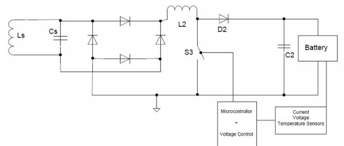
Figure 4 – Simplified Schematic of the Pickup Circuit.
