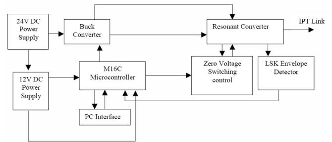
Figure 2 – Block Diagram of Charging Station
