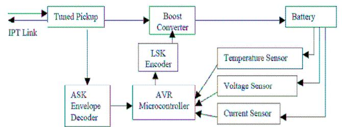
Figure 3 – Block Diagram of one Pickup
