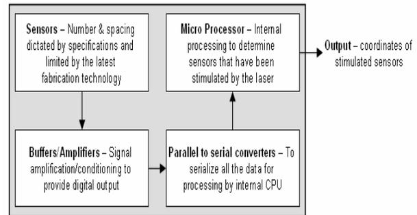
Figure 1 - Block Diagram of intended sensor system.
