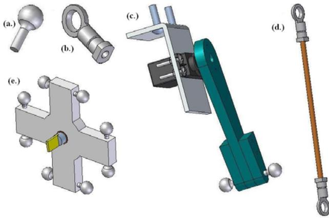
**Figure 2** - Significant mechanical parts that position the laser a. Ball from bearing b. Cup from modified bearing socket c. Servo motor with upper arm attached and mounting bracket d. Lower arm component e. Laser and laser mounting.
