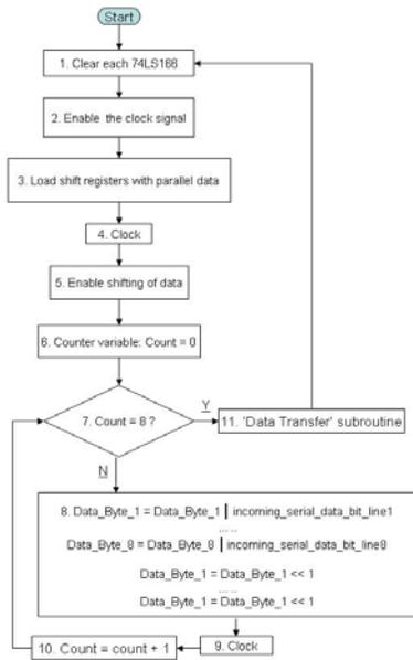
Figure 4 - Program flow for 'Data Acquisition'
