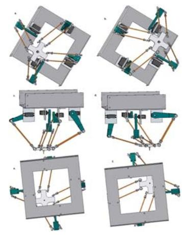
Figure 7- Simulation of laser tool head movement a,b Bottom views c,d Side views e,f Top views
