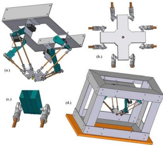
**Figure 3** - Assembly of all components resulting in the final structure a. All servos mounted with upper arm and lower arm attached to laser b. Lower arm attachment to laser end effector c. Articulated arm 'elbow' joint d. Complete Assembly.
