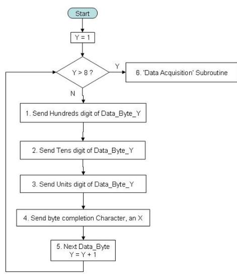
Figure 5 - Program flow for 'Data Transfer'
