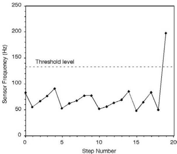
Figure 9 Tongue sensor readings during the spiral search.
