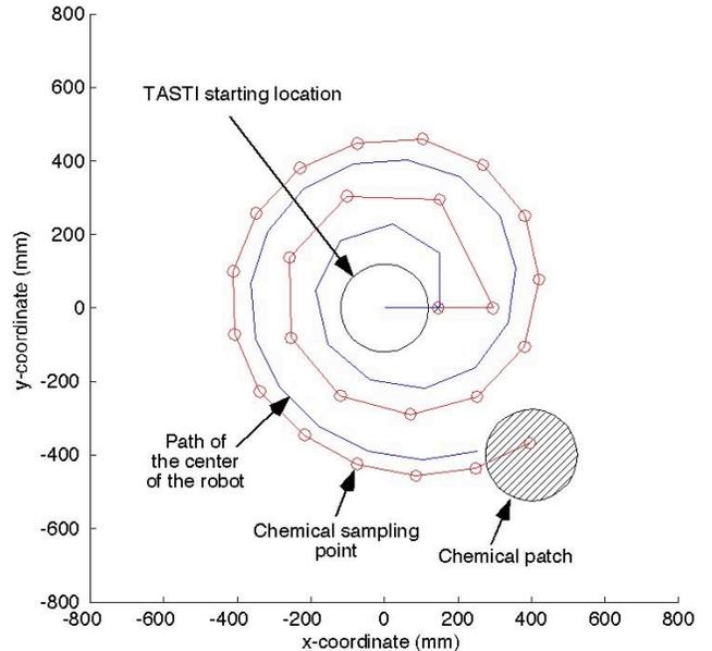
Figure 8 Spiral search path of TASTI the robot.
