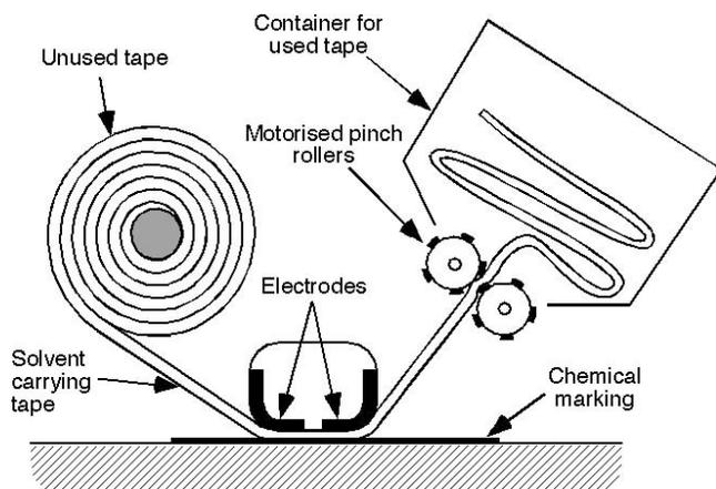
Figure 1 A schematic diagram of the robot tongue.
