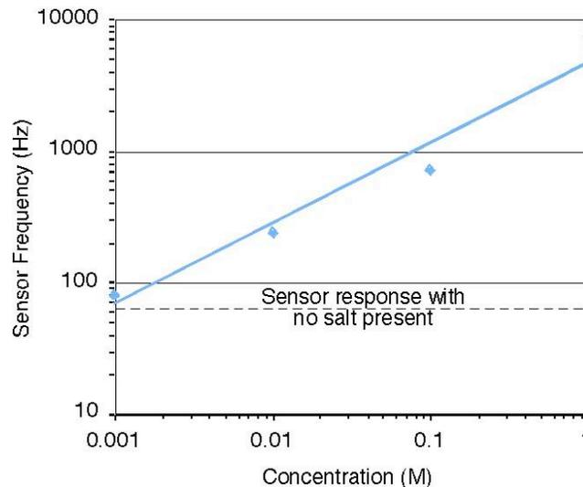
Figure 2 Sensor frequency related to chemical concentration.
