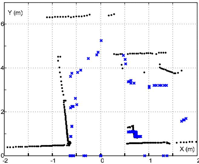
Fig. 9. Floor boundaries: crosses – stereo image based, dots – laser based
