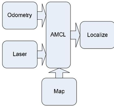
Fig. 10 input and output of AMCL
