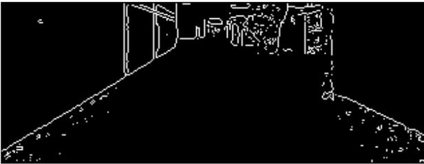
Fig. 4 Edge detection on subtracted image
