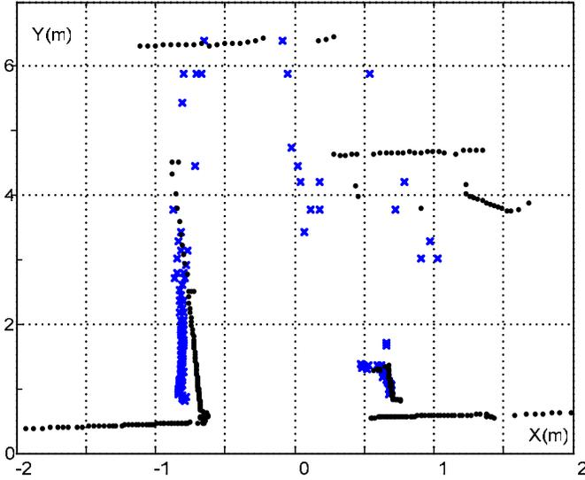
Fig. 8. Floor boundaries: crosses – image based, dots – laser based
