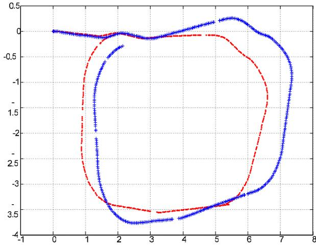
(a) Odometry (*crosses*) Vs True path (*dots*)
