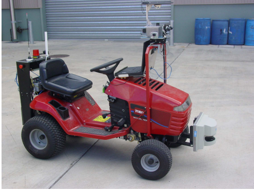
Figure 1: The experimental platform consisting of several cameras, GPS, IMU and laser rangefinder. At the rear of the vehicle are the vision processing and control computers.
