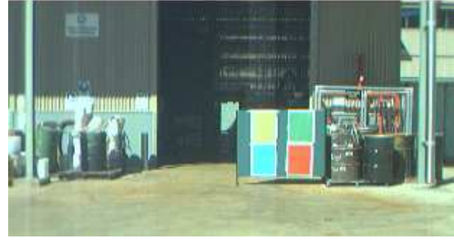
Figure 2: Yellow, green, blue and red targets taped onto a portable office partition at 9 m from the camera.
