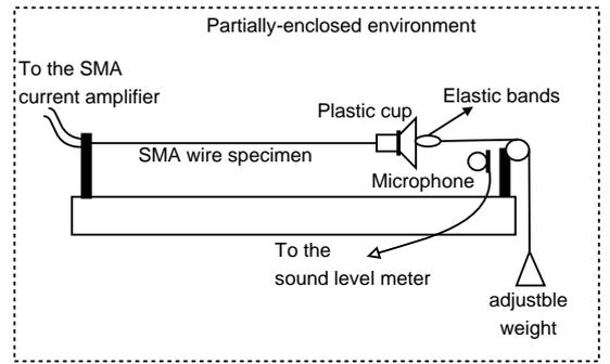
Figure 2: The schematic view of the loudspeaker setup
