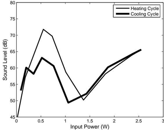
Figure 5: Sound level output from a normal Flexinol SMA wire using a 200 g load at 1000 Hz input signal.
