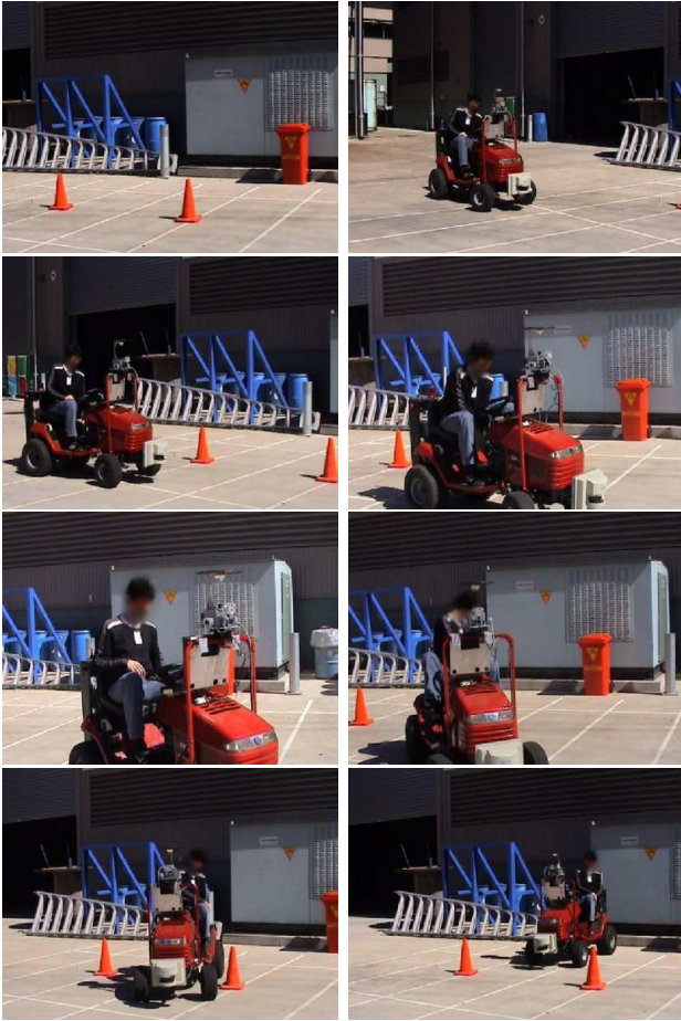
Figure 12: Sequence from a real parking manoeuvre: in this case the user only stays on-board for safety since no obstacle avoidance is active.
