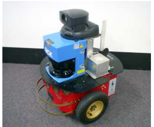
Figure 2: The Pioneer Robot with a SICK Laser, Sonar Ring, Active Camera and the EiMU sensor.
