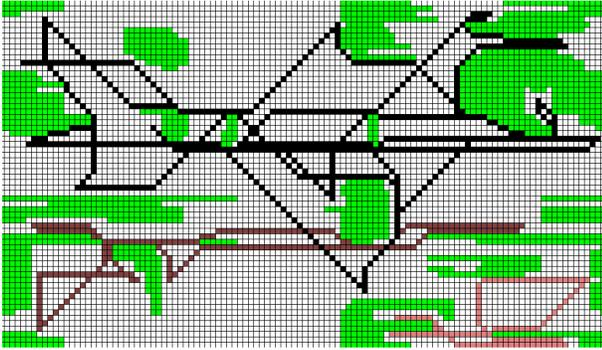
Figure 5: Trajectories of robots, optimal in path length.
