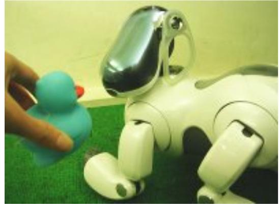
Figure 2: Waving an object before the robot so it can perform motion segmentation.
