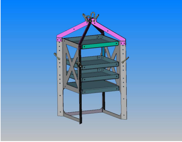
Figure 5: The pod for the AVS which carries the on-board computer and sensing.
