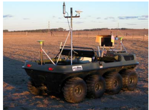
Figure 1: ARGO - an autonomous amphibious vehicle
