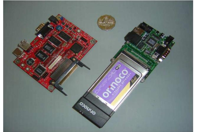
Figure 2: Typical sensor platforms. Stayton (left) and Star-gate (right)
