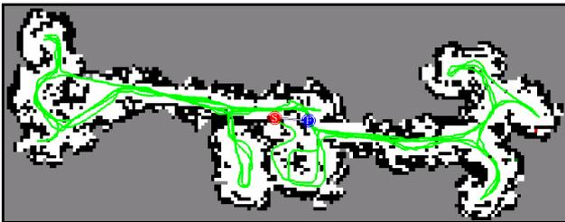
Figure 14 - Trajectory and occupancy map of the complete floor for  $\eta = 0.25$ . Note the consistency of the robot trajectory.
