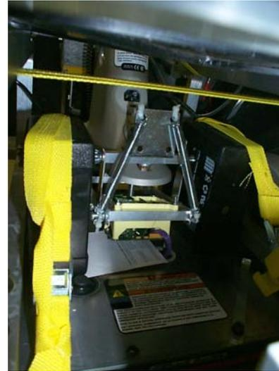
Figure 2: Tilt Sensor/Rate Gyro Assembly Control.
