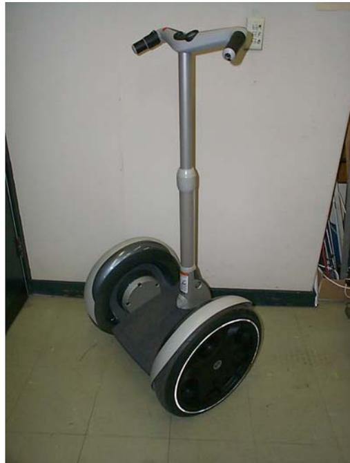
Figure 1. Segway Scooter for Personal Transport.
