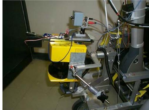
Figure 5: Gyro Stabilised Erwin Sick Laser Rangefinder with Tilt Control
