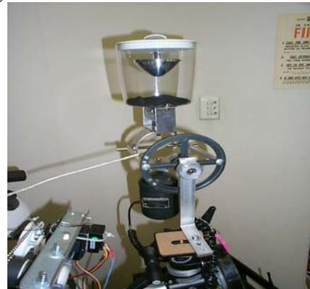
Figure 6: Gyro Stabilised Panoramic Mirror and Video Camera
