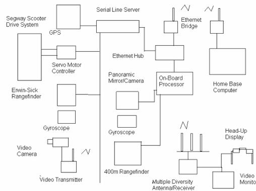
Figure 3: Instrumentation Schematic
