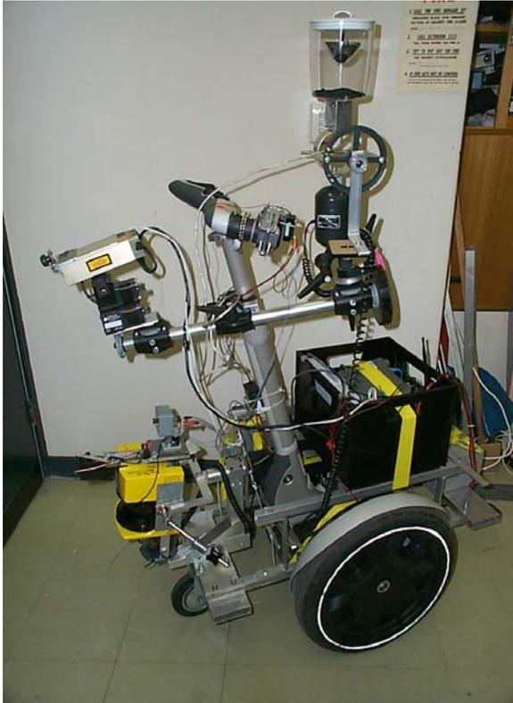
Figure 4: Robotically Instrumented Segway Scooter
