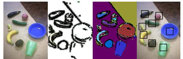
**Figure 6.** Result of online object recognition based on the genetically tuned parameters (from left to right): (a) original image frame (b) result of edge detection (c) tuned segmentation (d) object classification.
