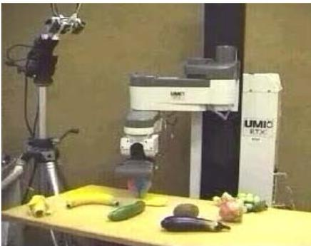
**Figure 7.** Table as a fixture that the objects are located on top of and the targets are within the robot's workspace (off-line table depth estimation).
