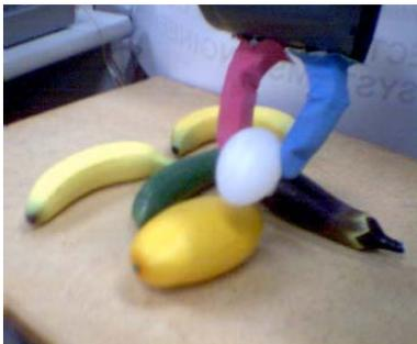
**Figure 3.** An egg is grasped and picked up by COERSU in a table-top scenario.
