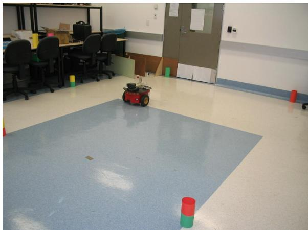
Figure 2: Pioneer 2 DXE robot in test environment. Note the coloured cylinders that are used as visual landmarks.
