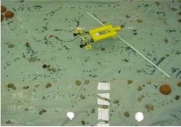
Figure 7: CSIRO AUV test tank with Starbug.
