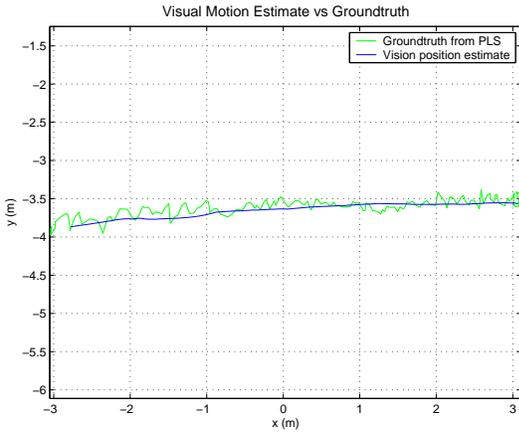
Figure 9: Position estimation using only vision and inertial information in short survey transect. Also shown is a ground truth obtained from the laser system.
