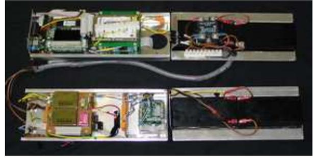
Figure 5: Starbug's sensing and computing instrument trays.
