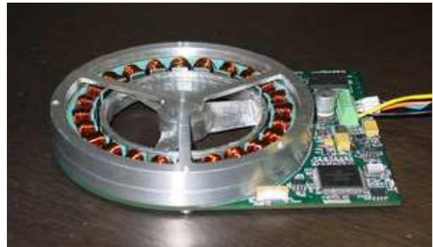
Figure 6: Novel low-profile manoeuvring "Flat thruster" designed for high torque and low drag.
