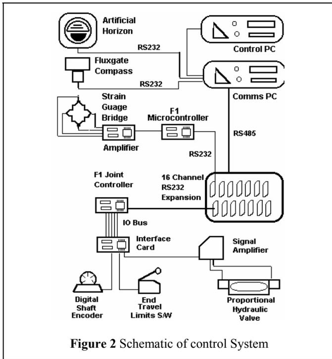
Figure 2 Schematic of control System
