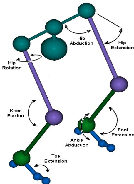
**Figure 1** Schematic of Roboshift showing degrees of freedom of the limbs.
