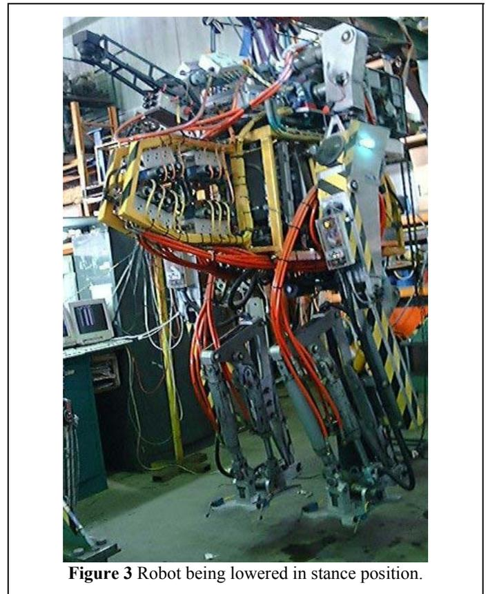
Figure 3 Robot being lowered in stance position.
