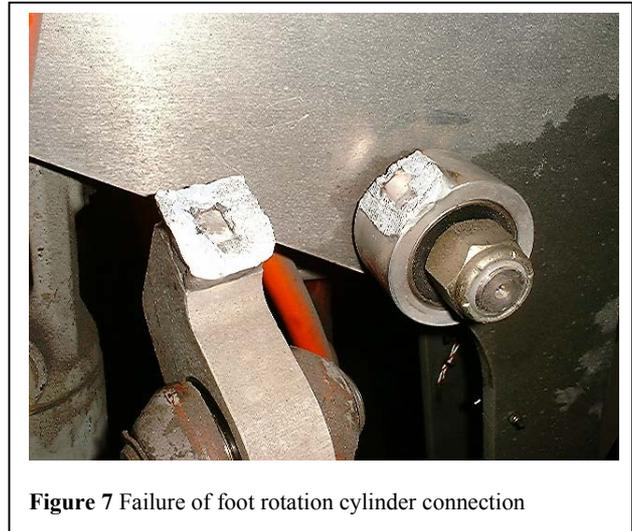
Figure 7 Failure of foot rotation cylinder connection
