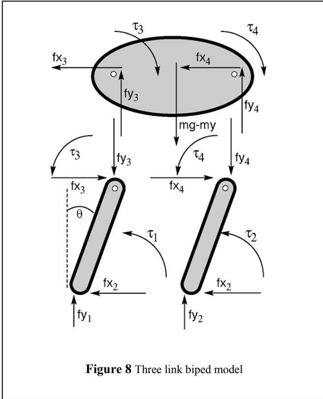
**Figure 8** Three link biped model
