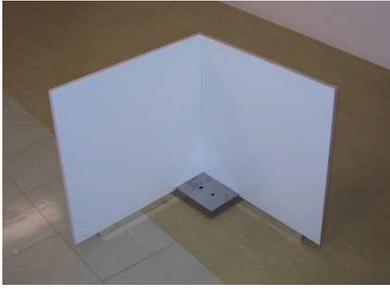
Figure 8: Laser calibration tool – “perfect” corner.
