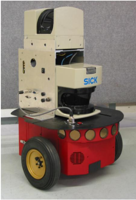
Figure 2: The 3D mapping robot. One laser range finder is used in the horizontal plane for providing location estimates. A second laser is oriented vertically to provide information for the 3D map building process.
