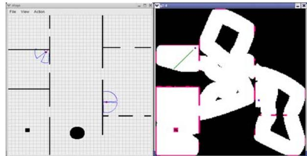
Figure 4 Simulated exploration of simple environment, actual map under Stage shown on left
