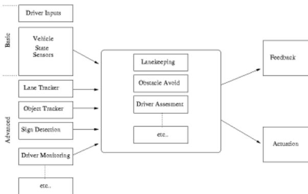
Figure 11: Subsystem interactions: The leftmost column represents system generalised sensors, including basic and advanced. The middle column shows desired behaviours and planning competencies for road or driver interactions. These in turn lead to outputs, the rightmost column.
