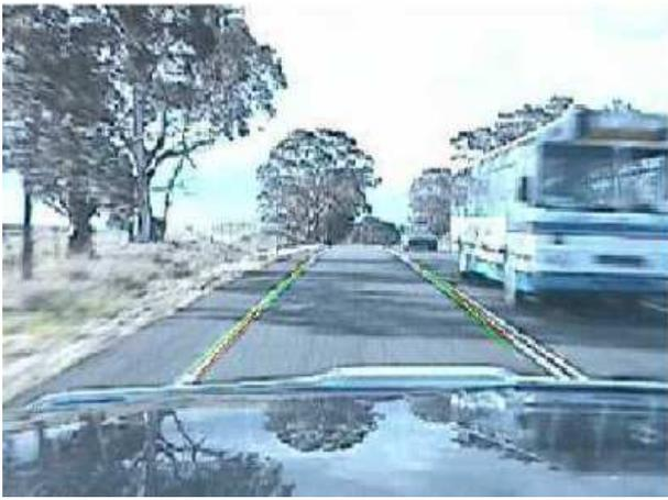
Figure 6: Lane tracker results. The coloured lines indicate the perceived lane position.
