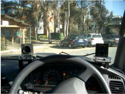
Figure 9: Facelab cameras mounted to observe driver.
