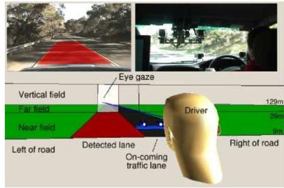
Figure 10: 3D model of how Facelab perceives the driver's head position and gaze. Additionally, top left inset shows results of lane detection, used to build Facelab world model; top right inset shows the scenario.
