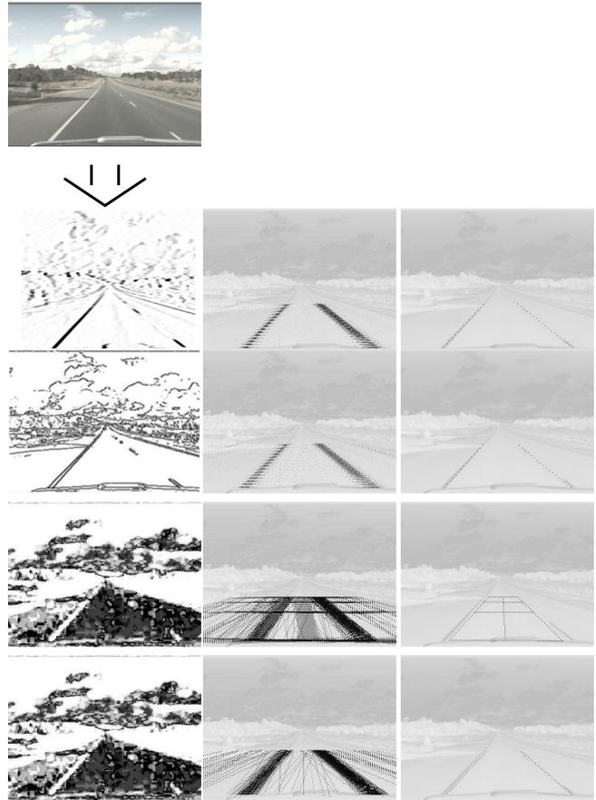
Figure 5: The top left image shows the video input to the lane tracker. The left column below shows preprocessed images which acts as input to the different particle filters. In the middle column, the current set of hypotheses are overlaid in image space. The most likely hypothesis, or particle, for each cue is then shown in the rightmost column. The order of the cues from top to bottom is: Lane Marker Cue, Lane Edge Cue, Road Colour Cue and Non Road Colour Cue.
