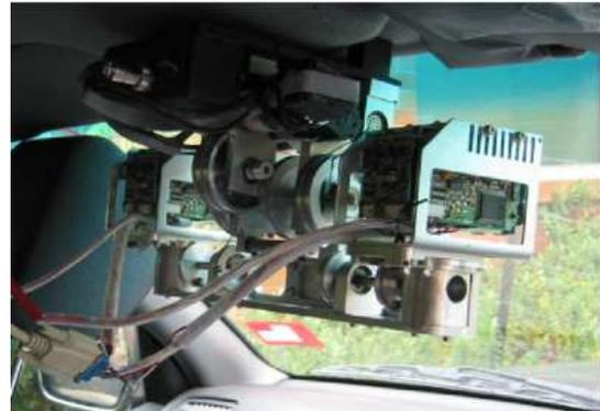
Figure 4: CeDAR mounted on the research vehicle.
