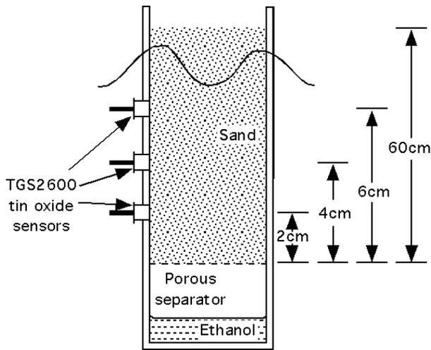
Figure 1 Experiment to estimate the rate of diffusion of ethanol vapour through dry sand.
