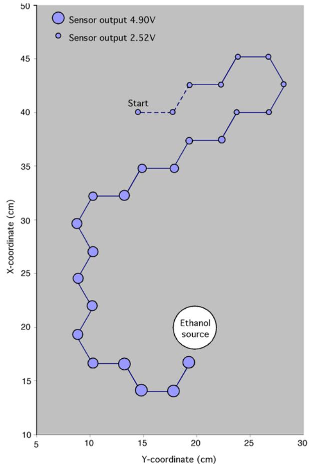
Figure 8 Experimental results of sensor probe path as the robot locates the buried ethanol source.
