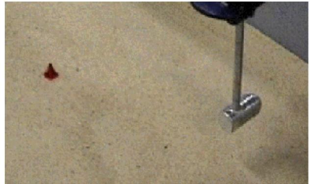
Figure 7 Chemical probe about to be inserted into the sand. The cone marks the position of the buried ethanol source.
