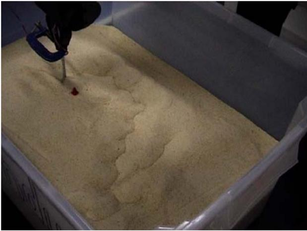
Figure 9 The experiment finishes when the probe collides with the ethanol source.
