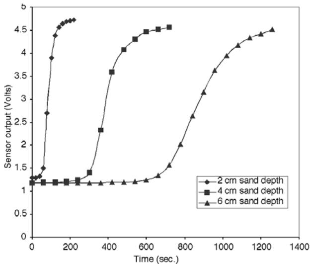
Figure 2 Diffusion of ethanol vapour through different depths of sand.
