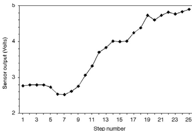
Figure 10 Gas sensor output voltage at each step in the source localisation procedure.
