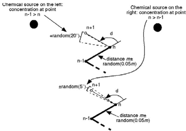
Figure 4 The *Planarian* algorithm modulates the turn angle based on readings of chemical concentration at points  $n$  and  $n-1$ .
