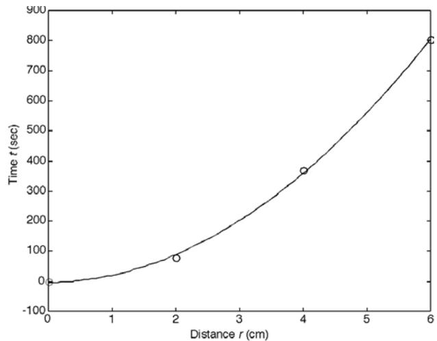
Figure 3 A plot of distance  $r$  against time  $t$  required for the chemical concentration to rise from zero to 15 ppm. The solid line represents the equation  $t = 22.1 r^2$ .
