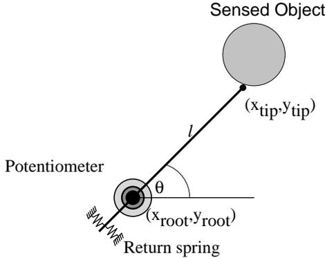
Figure 2: A schematic view of the whisker sensor.
