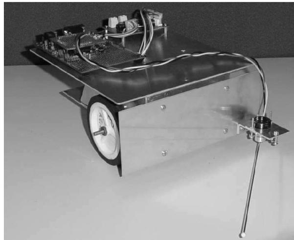
Figure 1: A whisker sensor based mobile robot.
