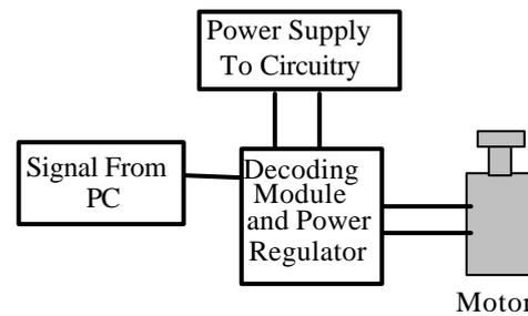
Figure 7. Analog signal decoding Module and Power Regulator.
