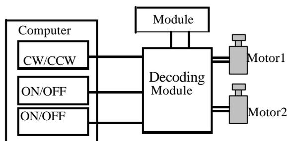
Figure 6. Digital Decoding Module and its Different Components.
