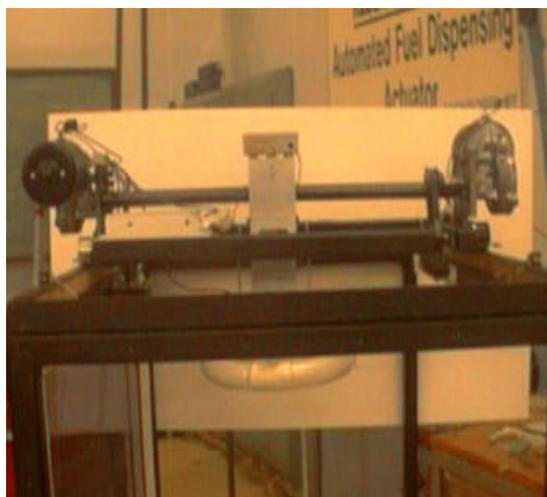
Figure 5. Camera Positioning Module with the Lighting Module.
