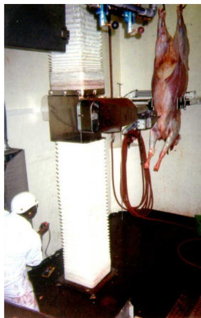
Figure 8: The world's first fully automatic brisket saw in action.
