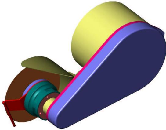
Figure 3. Robot mounted hide cutting tool.
