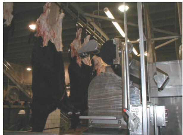
Figure 6: The beef belly rip robot in action.
