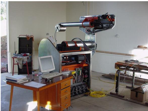
Figure 4: The partially assembled beef-processing robot.
