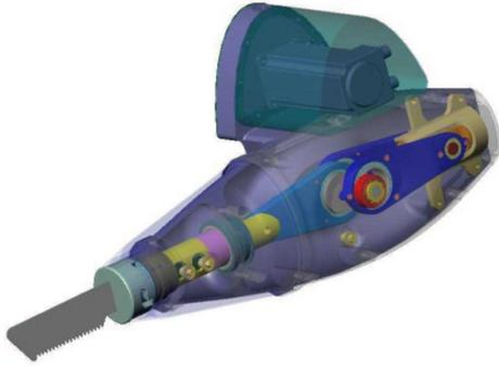
Figure 9: A Solidworks model of the briskeet-sawing tool.
